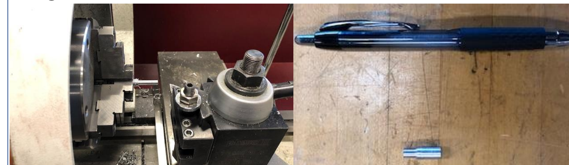
Figure 7: The aluminum inserts being turned on the lathe (left) and the inserts size compared to a standard pen (right).
