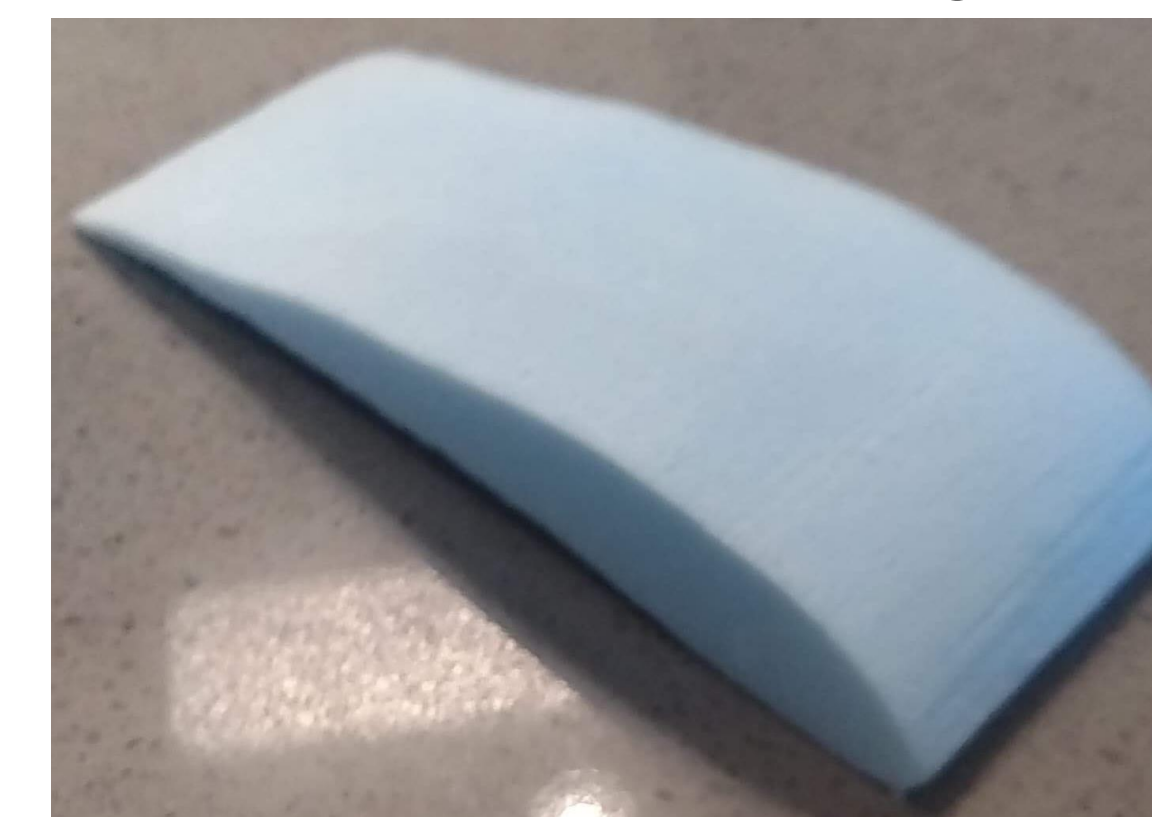
Figure 8: A 3" foam cut section of the S1223 airfoil.
