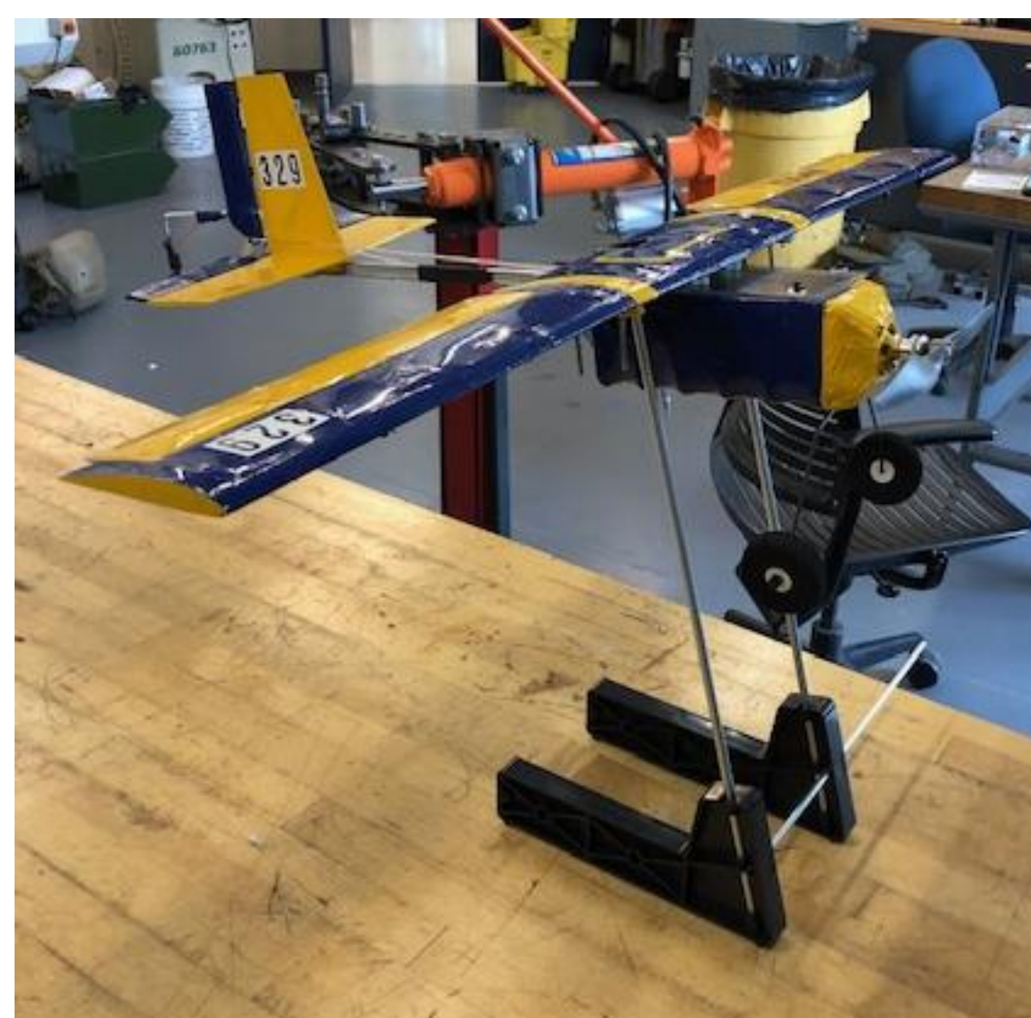
Figure 2: Center of gravity testing on the competition aircraft
